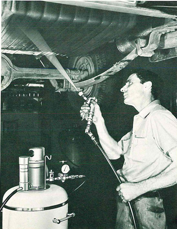
The spraying of undercoating is an added application of the air-motor type pump manufactured by Balcrank for the handling of greases and oils.
