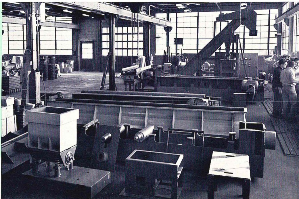
An inside view of the Plant No. 4 manufacturing facilities. Shown are Lorco Vibratory Finishing Machines in various stages of production.
